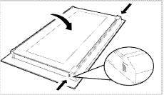
2. Pull the plastic component, attached on the upper section of the front door, towards yourself by simultaneously pressing on the pressure points on both sides of the component and remove it.
