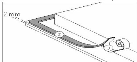
Stick the gasket (2) two millimetres from the external edge of the glass, after removing the protection tape (3).
