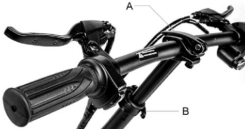
The angle of the handlebar can be adjusted by loosening the lever on the handlebar (A) and turning the handlebar up/down.
