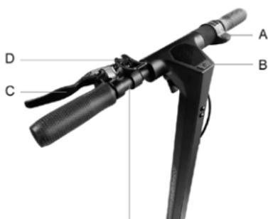
Throttle (A): press down to accelerate.
