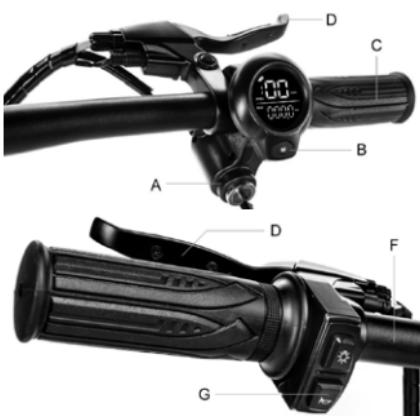
Ignition switch (A), to turn the display on/off, insert key into the ignition switch and turn the key to the right.
