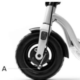
If the brake is too tight or too loose, adjust it by loosening or tightening the screw (A).
