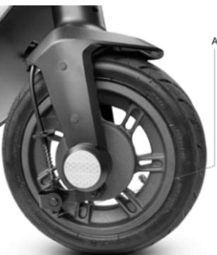
If the brake is too tight or too loose, adjust it by loosening or tightening the screw (A).
