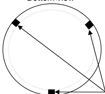
Put spacers in place under the glass before gluing it.
