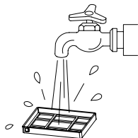
6. Gently clean the HEPA filter and the pre-filter with water.
