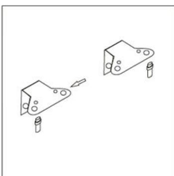
8. Raise the device and place the door on the bottom hinge. Check that the stem of the bottom hinge is inserted into the hole of the door. Then install the top hinge on the door. Before tightening the top hinge, try to open the door in order to check that the appliances closes hermetically. Then, screw the hinge cover onto the hinge
