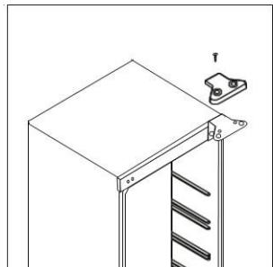
2. Open the door and unscrew the top hinge. Then lift the door to remove it from the appliance and put it on foam to avoid scratching and damaging it.
