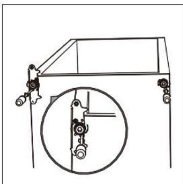
7. Unscrew the top stem and fit it on the left hole
